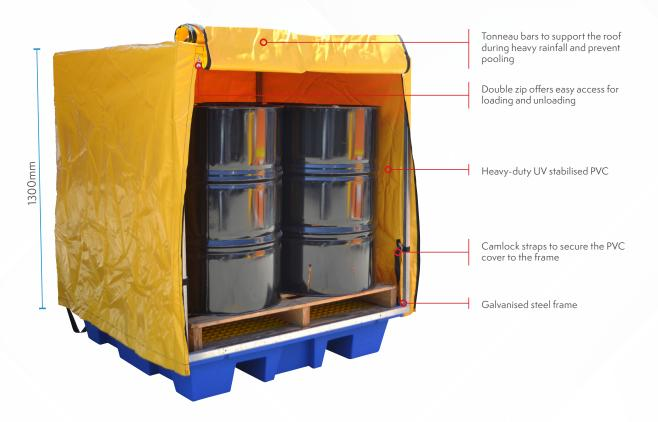
The 4 Drum Bund PVC Cover and Frame is a low cost option for turning your Bunded Pallet into an all-weather storage unit. It consists of a galvanised steel frame, heavyduty PVC cover with 2 zips and comes with complete instructions and fixings.
