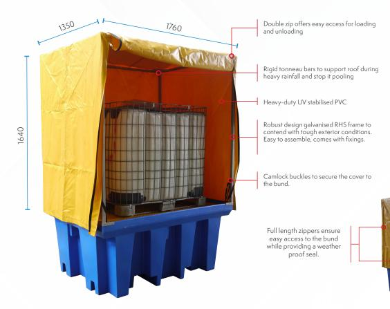
A robust and easily assembled weather cover to suit our Single IBC Bunded pallet. These units include a knock down galvanised steel frame which supports a heavy-duty PVC cover with twin full-length zippers to the front for quick and easy access.
