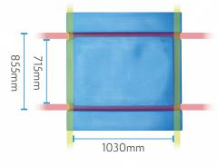
100 x 50mm bearers required to disperse storage weight to racking (can be supplied).
