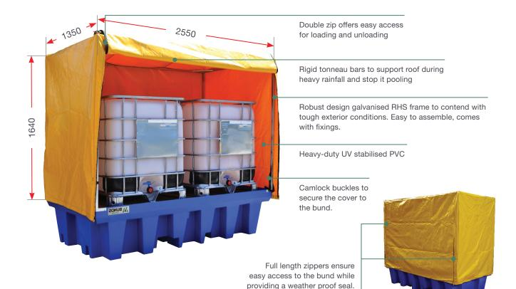
A robust and easily assembled weather cover to suit our Double IBC Bunded pallet. These units include a knock down galvanised steel frame which supports a heavy duty PVC cover with twin fulllength zippers to the front for quick and easy access.
