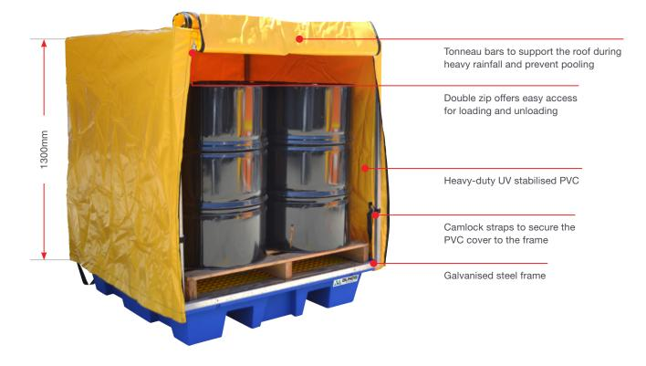
The 4 Drum Bund PVC Cover and Frame is a low cost option for turning your Bunded Pallet into an all-weather storage unit. It consists of a galvanised steel frame, heavy-duty PVC cover with 2 zips and comes with complete instructions and fixings.
