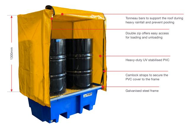
The 2 Drum Bund PVC Cover and Frame is a low cost option for turning your Bunded Pallet into an all-weather storage unit. It consists of a galvanised steel frame, heavy-duty PVC cover with 2 zips and comes with complete instructions and fixings.
