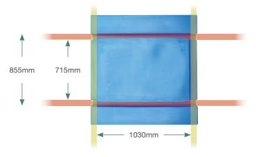
$100 \times 50 \text{mm}$  bearers required to disperse storage weight to racking (can be supplied).
